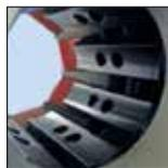
With the double pin connection, it is possible to crimp on the front and rear sides of S3 series machines. (not the light model)
